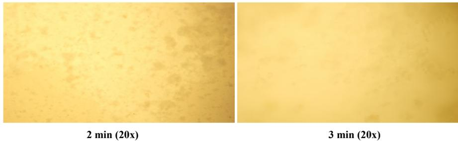
Figure 2 Optical micrograph view of Cp-Ti plate coated with nano HA and MgCl<sub>2</sub> using 30 V in different times (20x)
