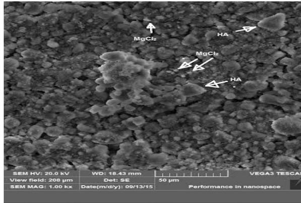
**Figure 4 SEM Images surface morphology of coated specimens (HA/MgCl<sub>2</sub>)**
