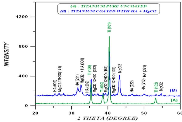
Figure 1 X-ray diffraction patterns of coated and uncoated specimen
