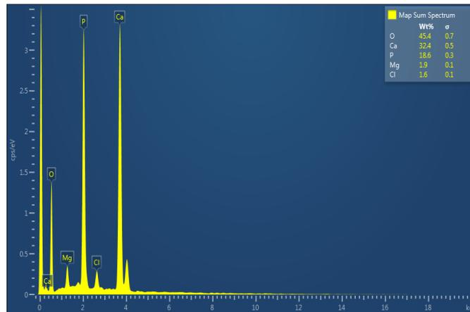
**Figure 5 EDX image of elements coated Cp-Ti specimens (HA/MgCl<sub>2</sub>)**
