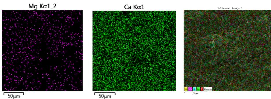
**Figure 6 EDX map of the composition of coating materials HA/MgCl<sub>2</sub>**
