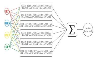
Figure 1 Proposed architecture of the preterm monitoring system
