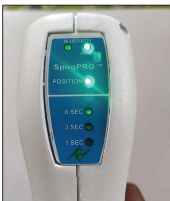
Figure 3 SpiroPRO™ LED indicators for correct positioning and maneuverer progression
