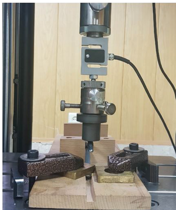
Figure 2 Constructed debonding apparatus
