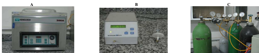
Fig 1.(A) Modified atmosphere packaging, (B) gas analyzer, (C) gas flash tank(Model: Boxer-200A) [15, 25-28]
