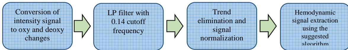
Figure 7: The block diagram of signal preprocessing steps
