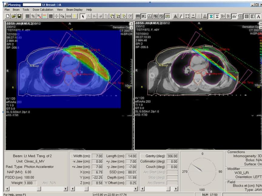
Figure 2 Radiation beam and wedges application to PTV and 2D dose distribution with iso-dose lines
