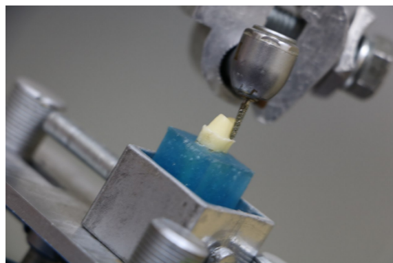
Figure 1 Instron test machine with modifications for testing
