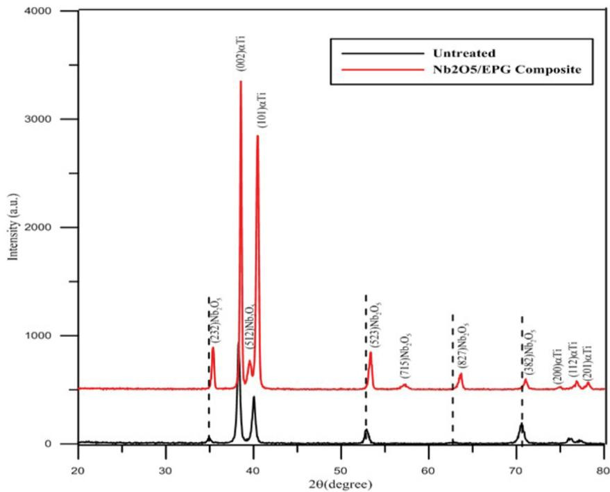
**Figure 6 XRD patterns of CPTi substrate coated with Nb<sub>2</sub>O<sub>5</sub>/PEG composite**
