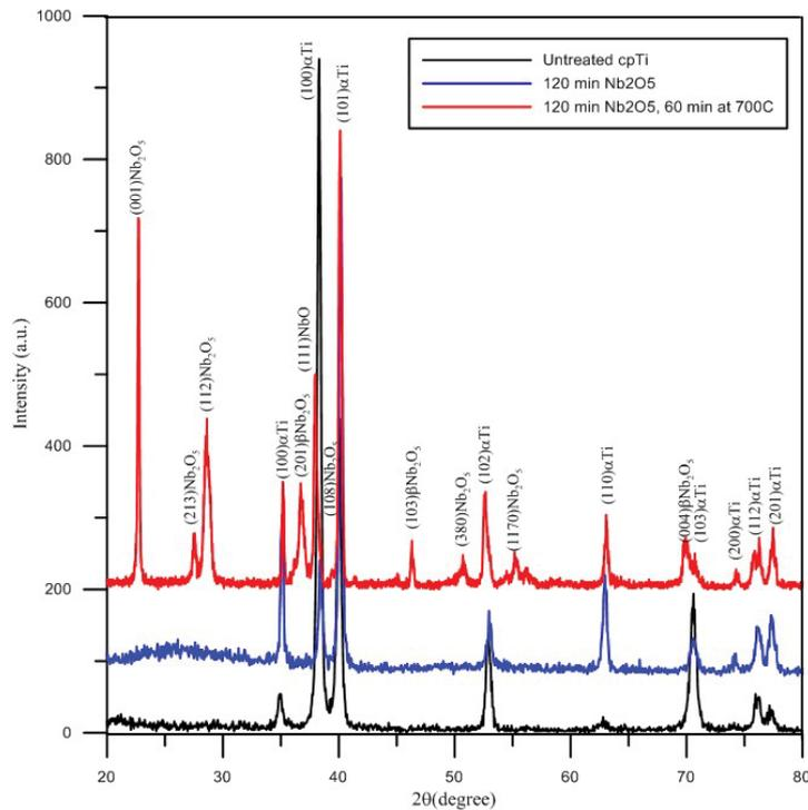
Figure 5 XRD spectroscopy of  $Nb_2O_5$  coating at 120 min magnetron plasma sputtering
