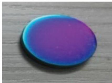
Figure 2  $\text{Nb}_2\text{O}_5$  coated CPTi disc
