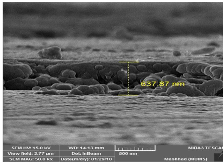
Figure 8 SEM micrograph demonstrated Nb<sub>2</sub>O<sub>5</sub>/PEG biocomposite film thickness
