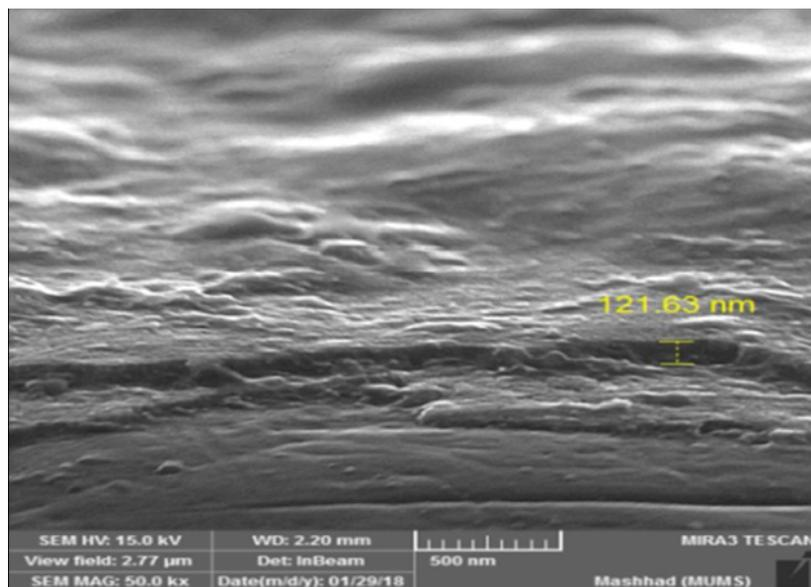
**Figure 7 SEM micrograph demonstrated Nb<sub>2</sub>O<sub>5</sub> coat thickness**
