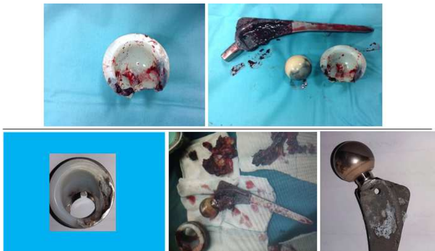
Figure 3. Corrosion in prosthetic femoral component, the polyethylene liner and the exterior of the metallic head; lower pictures are related to case 2 and upper case 1
