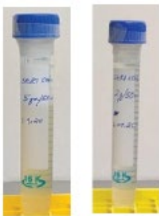
Figure 5 Extracted sericin concentration (A) (5 g/50 ml DD H 2 O) (B) (2 g/50 ml DD H 2 O)
