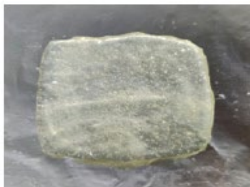
Figure 6 Sericin gel before drying
