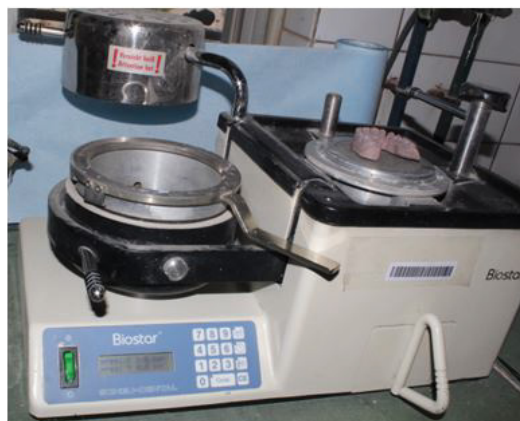
Figure 2 preparing the Biostar machine for the thermofforming process with the model centered on the working bench of the machine
