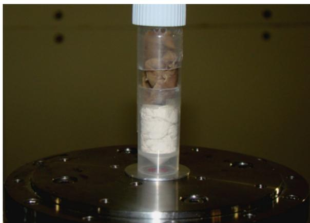
Figure 1 Liver sample of rat mounted in plastic vial with a transparent region for synchrotron beam
