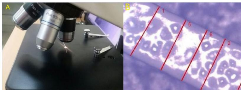
**Figure 1 (A) Wire segment under microscope lens; (B) Wire as it appeared in the computer display**
