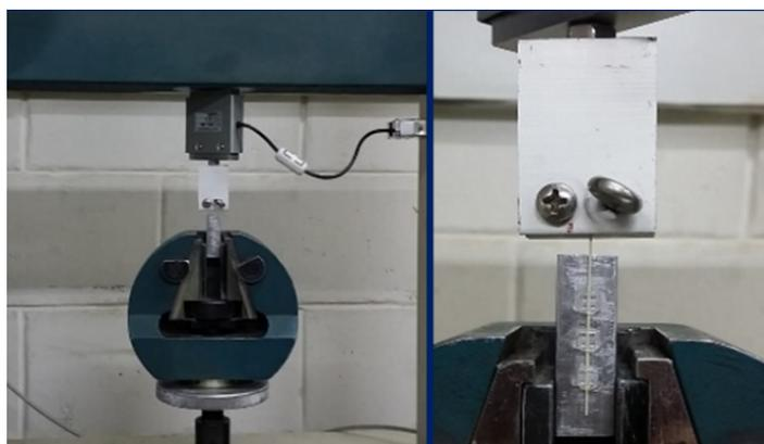
**Figure 3 Wire-bracket-block system fixed to machine**
